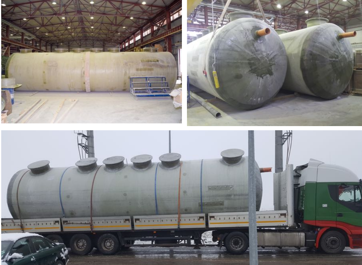
Fig. 49 GRP biological modules
